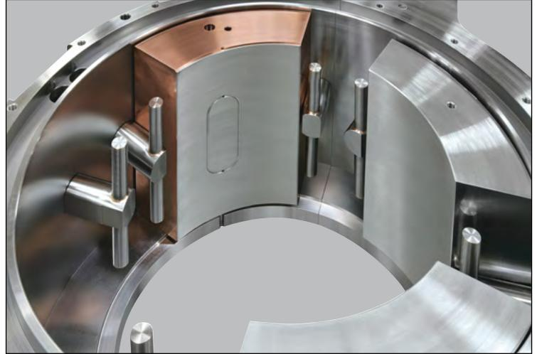
Hydrostatic jacking grooves in the lower pads not only reduce friction during start up but increase safety margins and machine reliability. The bearing also includes a provision for instrumentation to match original equipment fittings as well as the ability to directly measure electric resistance of each insulating layer when assembled.
