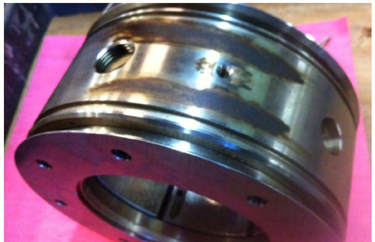
*Figure 3: Damage on the OEM bearing outer diameter from bottoming out*
