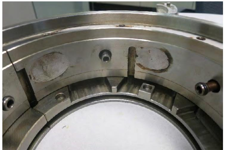
*Figure 2: Pivot wear on the point-contact-pivot tilt pad (top) and bearing shell bore (bottom)*
