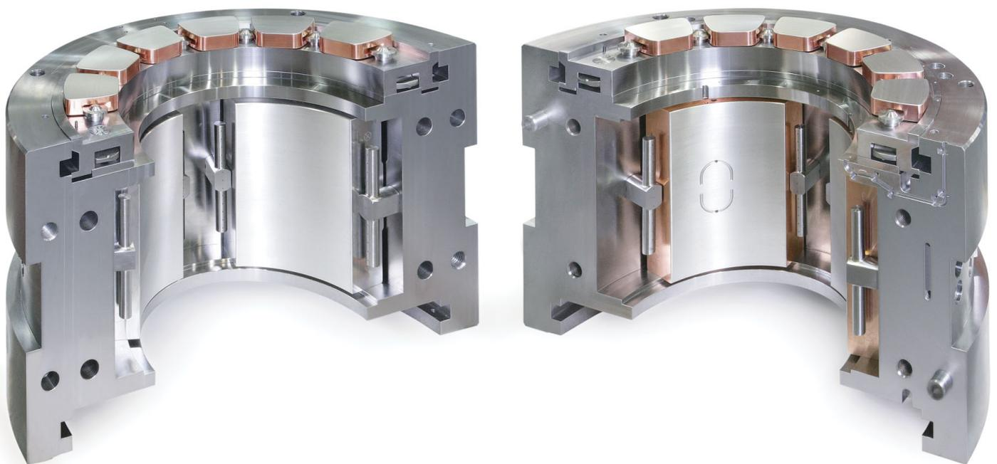
*Maxalign bearing using a combination of standard whitmetal lined steel backed pads and whitmetal lined copper chrome backed journal pads with hydrostatic jacking; combined with copper chrome backed thrust pads*
