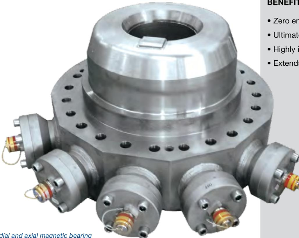
*Radial and axial magnetic bearing stators with position sensors integrated into a hermetically sealed housing for a vertical, integrated motor-compressor application.*
