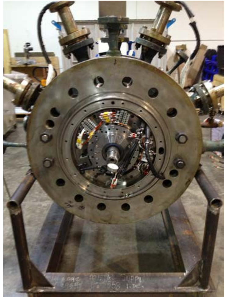
Figure 5: Replacement radial AMB hardware, including the stator, position sensors and speed sensors
