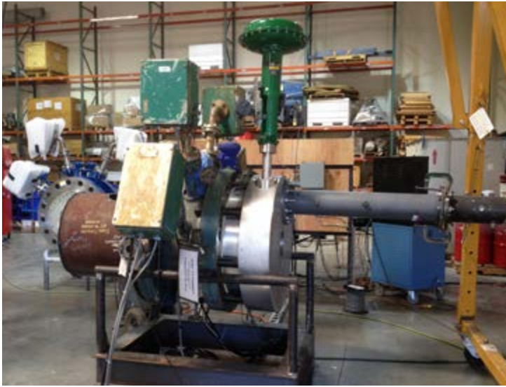
Figure 2: Turboexpander unit prepared for commissioning and testing at L.A. Turbine's test facility
